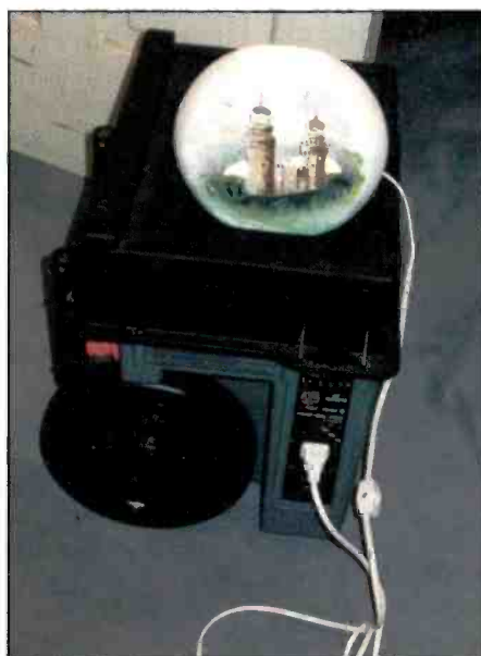
Given a full charge, you'll have plenty of light from a small lamp. The 1500 provided us with light for about eight hours from a 40-watt lamp, but use a smaller bulb, say 25-watts, and that eight hours could easily be 20.
